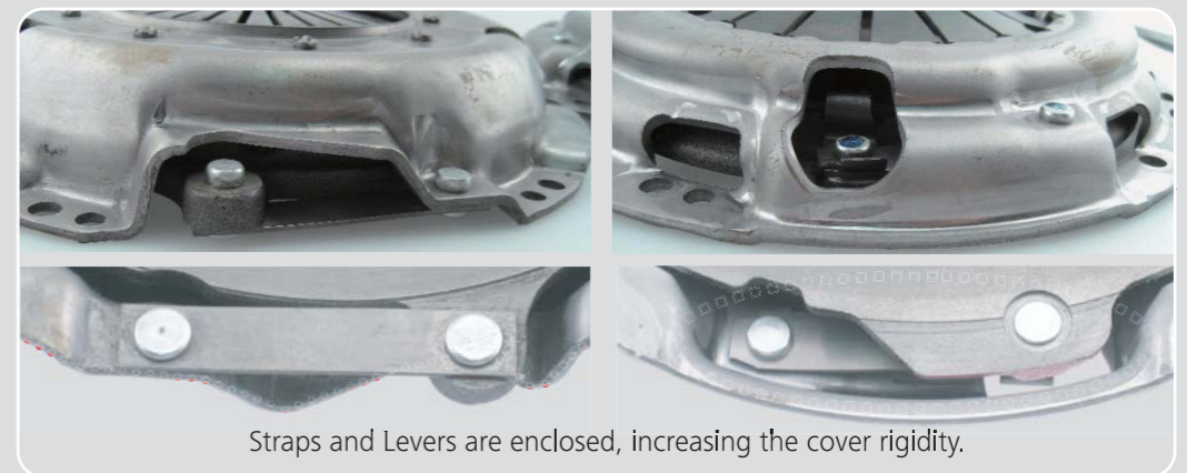
NVR Covers have fewer Fingers, but the Diaphragm Spring Fingers are thicker and stronger .
